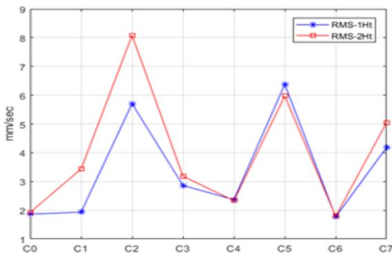
Fig 5: Variation of RMS for horizontal directions of two bearing-1500rpm
