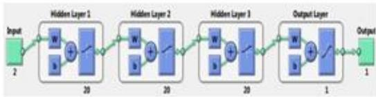
Fig 6: Feed forward BPNN architecture
